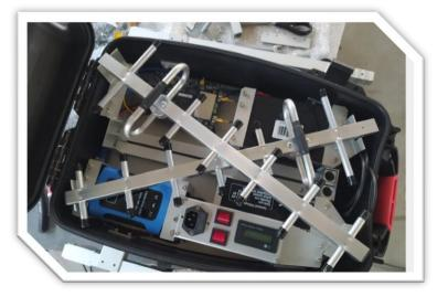
The backpack contains the battery charging system and a control panel, as well as the electronics.
